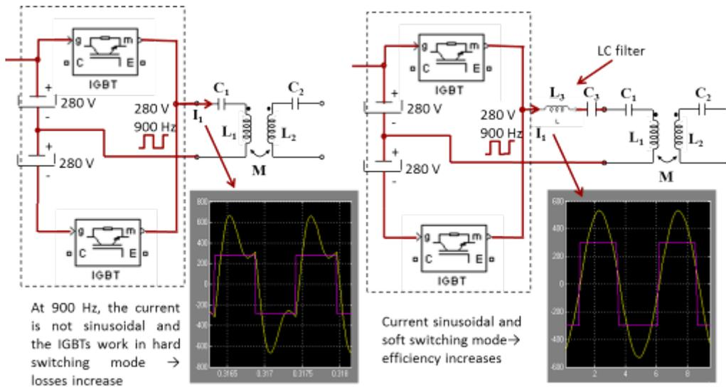
Figure 2: Electrical designs to adapt the wave form induced in the IPT system and wave used for the heating coils.
