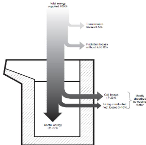
Figure 3: Main energy losses on an induction heating system
